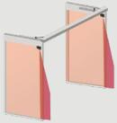
The LZR<sup>®</sup>-FLATSCAN SW is a safety sensor for automatic swing doors based on laser technology. It secures the moving door wing as well as the hinge area. To do so, a module must be installed in the upper corner of the door wing on both sides of the door.
