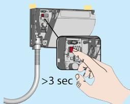
The service mode deactivates the safety detection during 15 minutes and can be useful during an installation, a mechanical teach-in of the door or maintenance work.
